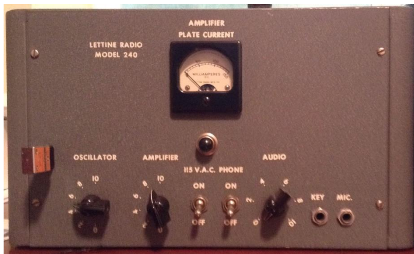
KN7SAI transmitter - 17 watts output!
